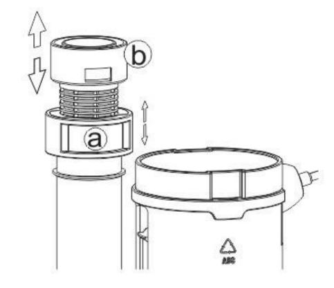
6. To adjust the height of the overflow pipe, slide the lock (a), then set the desired height of the overflow pipe (b). Put the lock back after.
