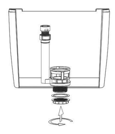
3.Insert the flush valve's base into the water tank. Screw on the nut collar and hex nut properly.
