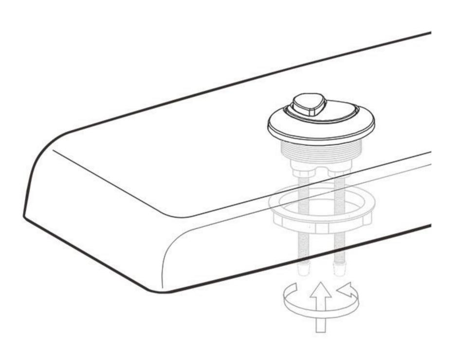
2.Insert the button into the hole on the water tank. Screw the nut.
