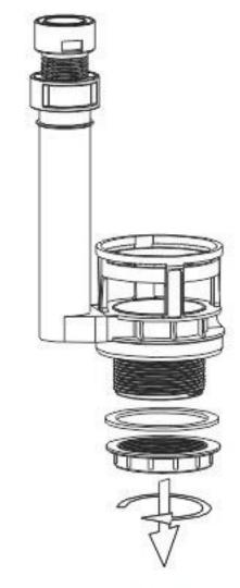
2.Remove the hex nut and nut collar from flush valve base.Don't remove the seal !!!
