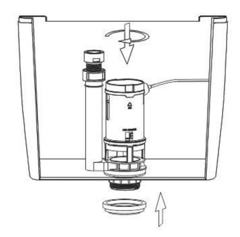
4. Take the body of flush valve and set it into the base and lock in place by rotating it clockwise. Then Insert the tank to bowl rubber gasket on to the flush valve's outlet bottom.
