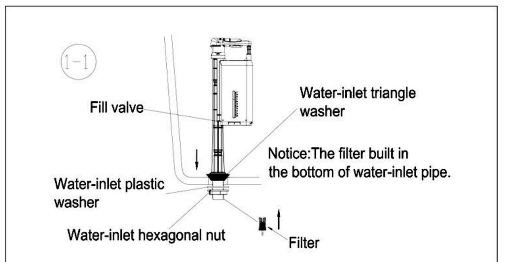
Put fill valve & water-inlet triangle washer insert into water-inlet hole of water tank, then, cover water-inlet plastic washer and hexagonal nut in turn from the bottom of fill valve. Fastening water-inlet hexagonal nut and make a proper adjust according to the size of water tank.
