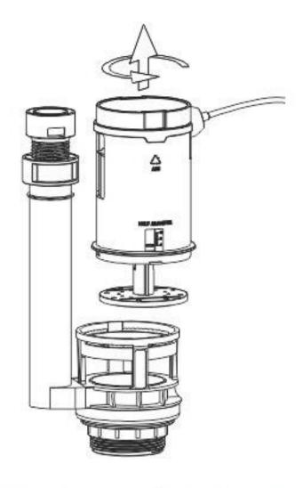
1.Hold the base of the flush valve and rotate the body counterclockwise take it out of base.
