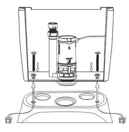
5. Fasten the tank to bowl with one pair of plastic or stainless steel bolts. Make sure bolts have the black rubber washer under the bolt's head.
