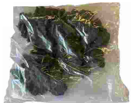
Bag of Ceramic Shale – to be laid on the Burner Grate
