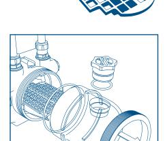
Remove dome from base, empty exhausted Combiphos and clean base. Fit new 'O' ring seal, refit dome and aluminium ring. Refill with new Combiphos
