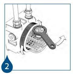
Place a bowl under unit to catch any residue. Unscrew red filler plug using the spanner provided. Unscrew and remove aluminium ring.
