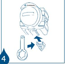
Refit red filler plug and replace front cover. Hang spanner on hook.
