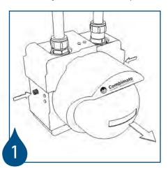
Depress the two red buttons and pull the cover away from the unit (Water flow through the unit is shut off when the cover is removed).
