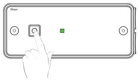
When the LED stops flashing red, release the Set button. The LED stops flashing upon successful reset of the Relay.
