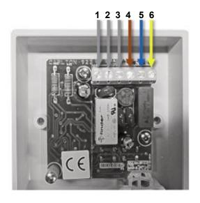
From Left to Right terminals 4-6 correspond to the Mains cable wires.
