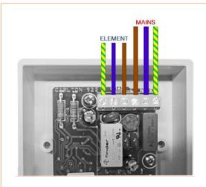
Clamp the element cable to the bottom of the wall controller
