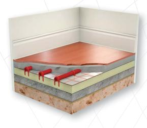
The pipe is positioned in place and then a barbed Tackernail is fixed over the pipe by means of a MYSON FLOORTEC Tackertool 3D. The barbs snag on the foil material holding the pipe until the screed or concrete is laid.
