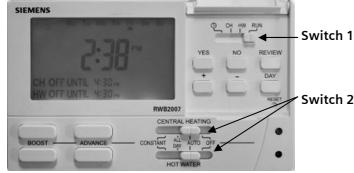
**Switch (1)** Programming switch. When all programming has been done this switch must be in Run
