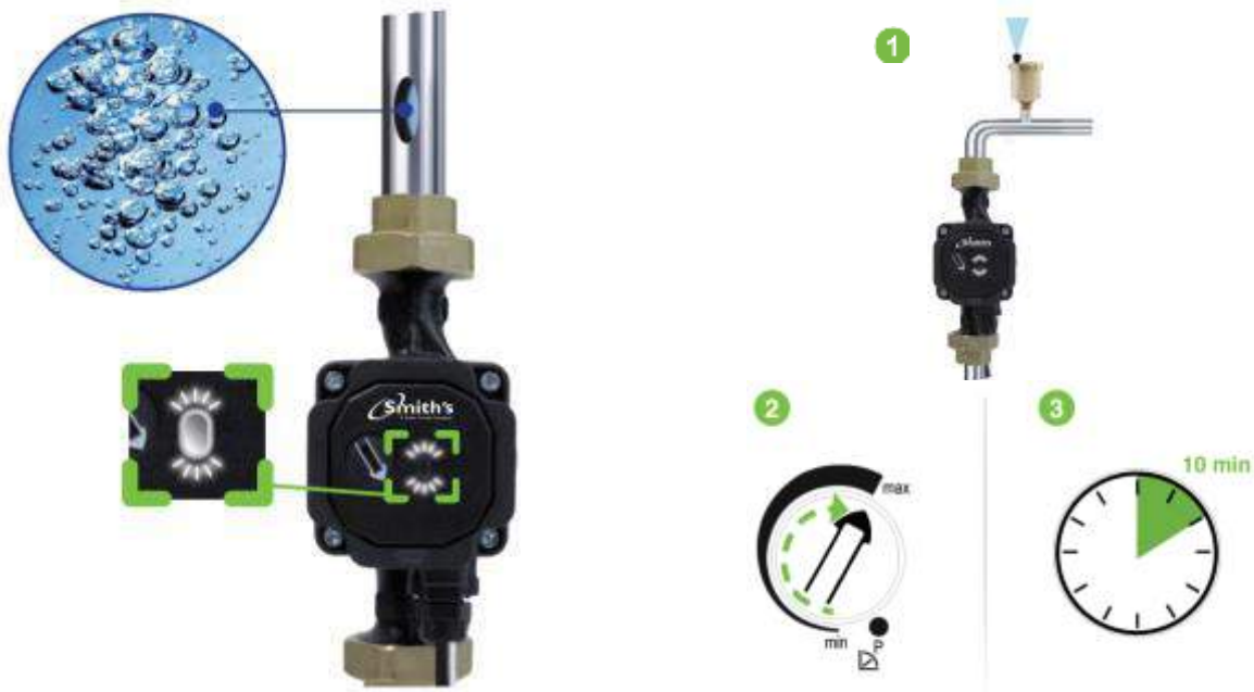
Fig. 9.2: Filling and venting of heating systems
